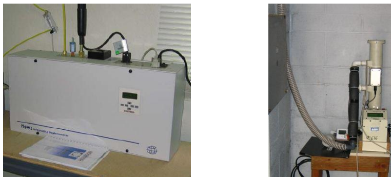
Figure 6. Ecotech Nephelometer shown on left, and Radiance Research shown on right.
