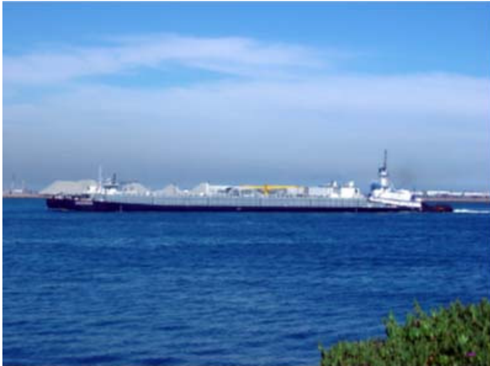
Figure 3.10: Integrated Tug and Barge
