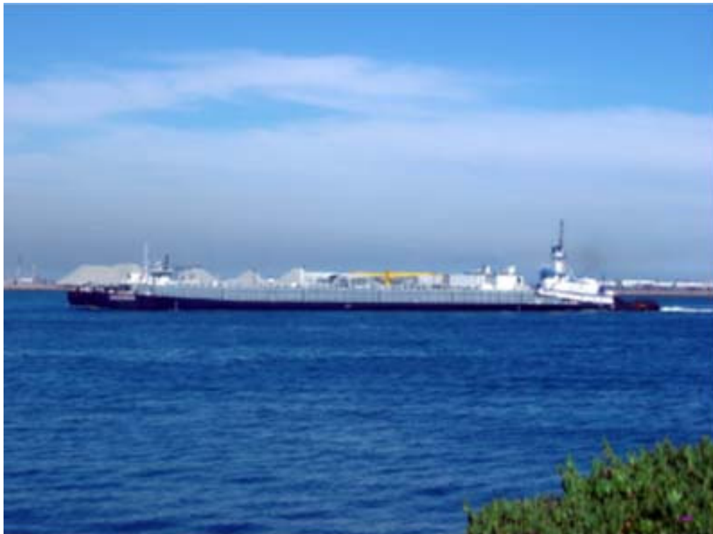
Figure 3.10: Integrated Tug and Barge
