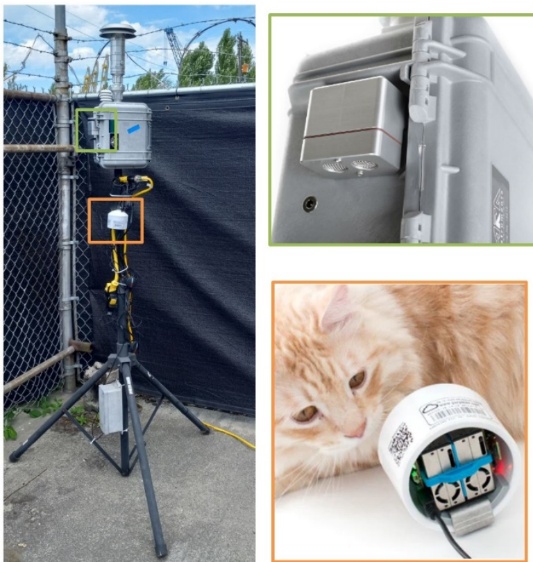
Figure G-1: illustration of the N-FRM installation at our UEWA (Fontanelle St.) site, with Purple Air sensor added to the setup(left). The other two photos (borrowed from Purple Air© and ARA instruments© websites), provide a more detailed look at the N-FRM RTP (upper right) and Purple Air sensor (lower right).
